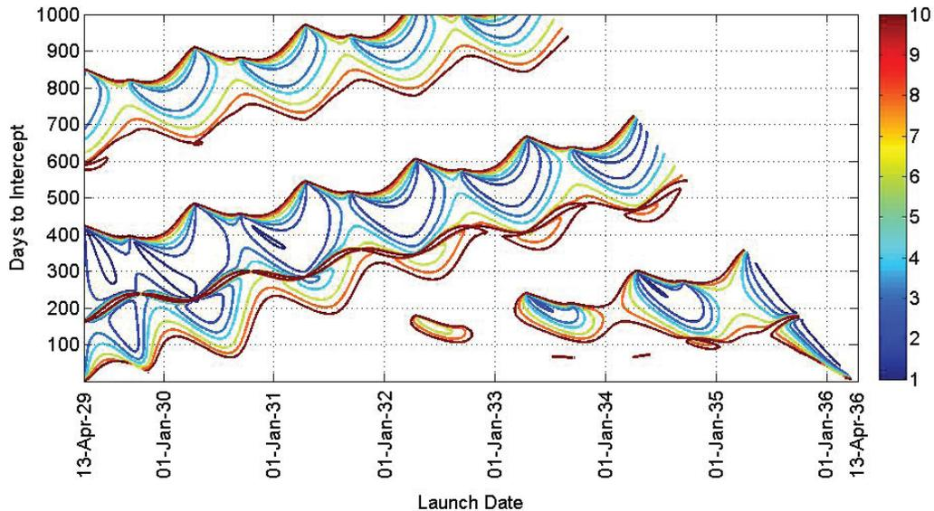
Figure 3. Direct Intercept Porkchop Plot Showing  $\Delta V$  Requirements vs. Transfer Time
