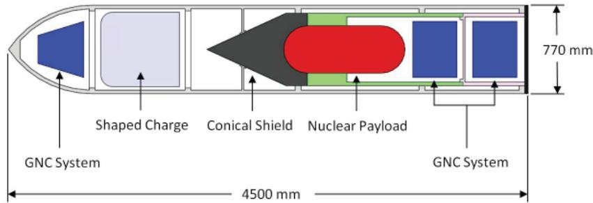
Figure 6. NED Variant-1 Internal Component Breakdown
