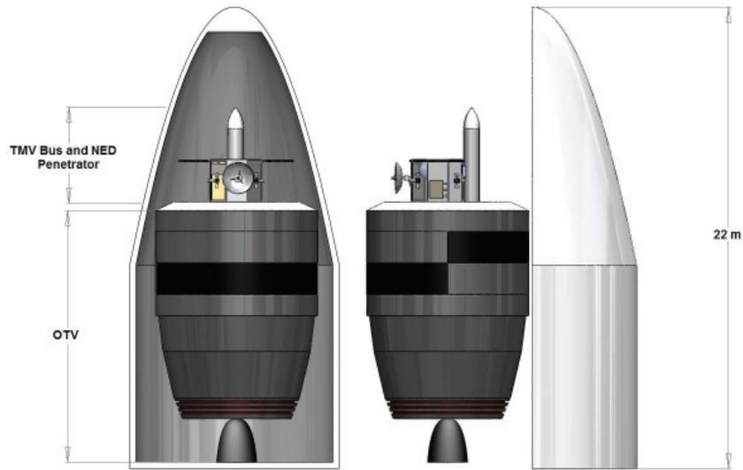
**Figure 7. Illustration of Possible IPBM Configuration Insided an Ares V Fairing**
