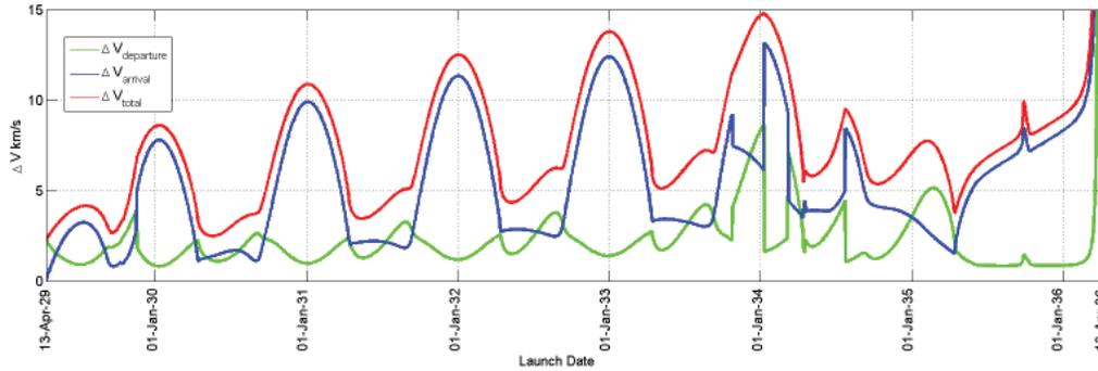
**Figure 1. Minimum  $\Delta V$  Requirements From 2029 to 2036**
