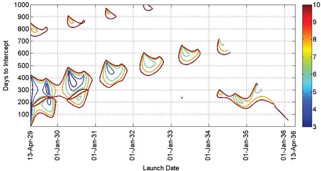
Figure 2. Rendezvous Porkchop Plot Showing  $\Delta V$  Requirements vs. Transfer Time
