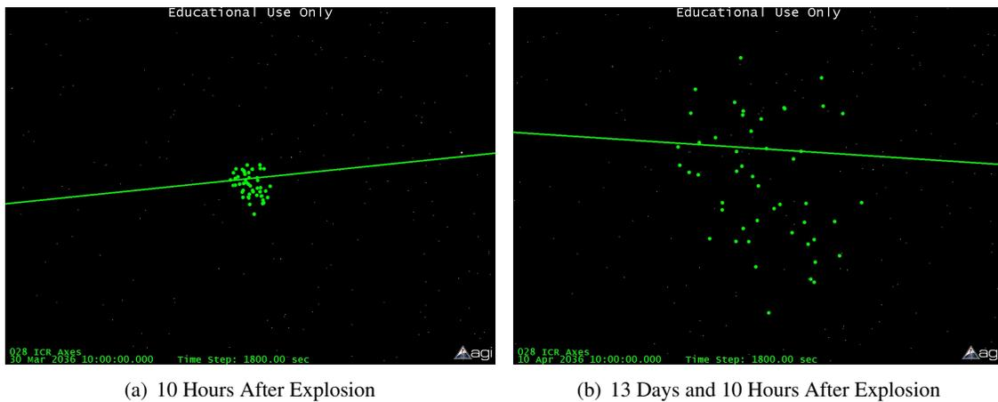
**Figure 7. Orbital Dispersion of Fragments after Nuclear Explosion of Apophis.**
